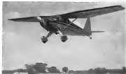
Dallas-Dall Four-Placer —First flight picture of the new four-place all-metal Weatherly-Campbell 140 hp personal plane, built in Dallas, Tex., shows compact taper wing, strut-braced fuselage, landing gear track, and general conventional lines of plane.
